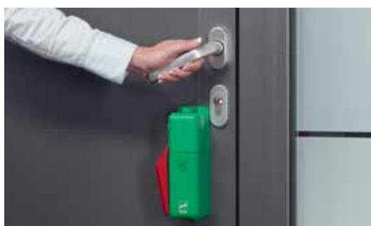
The door can be opened in an emergency by using the door handle. If opened, the surveillance lever is activated and an audible alarm is sounded, which can only be reset using the integrated locking cylinder. The surveillance lever swings downwards if the door is opened, thus also giving visual indication that the alarm has been triggered.
