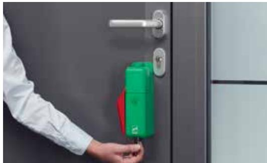
The surveillance alarm can be deactivated by the profile cylinder. The surveillance lever is secured in the lower position. The door can now be opened using the door handle without triggering the alarm.
